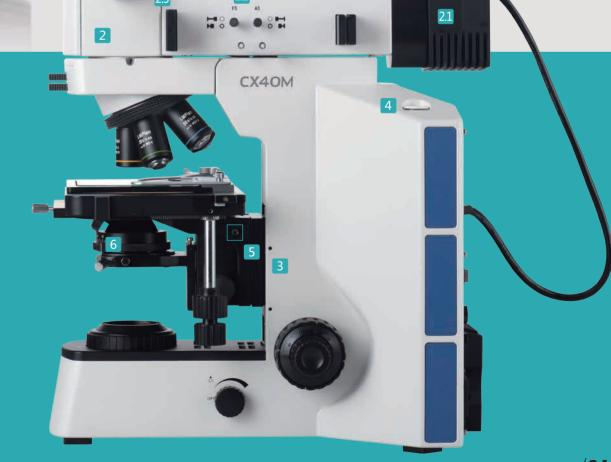
Bright field, oblique light and simple polarizing are all available with CX40M. Brightfield image with high brightness and high resolution shows original color of samples. And oblique light is used to show 3D relief image.
